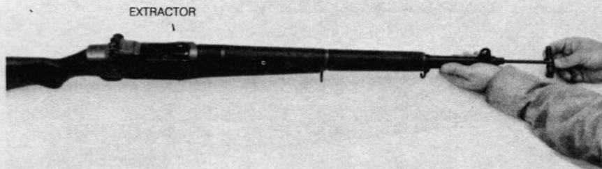
Figure 14. Removal of ruptured cartridge case.
