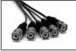
*BNC Connectors:* Another type of input that is found on many display devices is the BNC connector. There are usually either 3, 4 or 5 BNC connectors depending on how your display device handles synchronization signals. These connectors are used on higher-end TVs, monitors and CRT projectors. These connectors are most commonly used for RGB but are sometimes used for Y-Pr-Pb signals as well.
