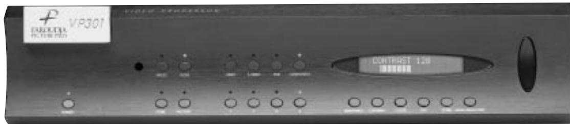
The Faroudja VP301 Line Multiplier is a precision video instrument used to convert NTSC interlaced signals into 600 visible, progressively scanned lines (800X600 resolution). Using Picture Plus™ technology, the VP301 removes typical video processing artifacts while also increasing color purity and image detail, closely matching 35mm film.
