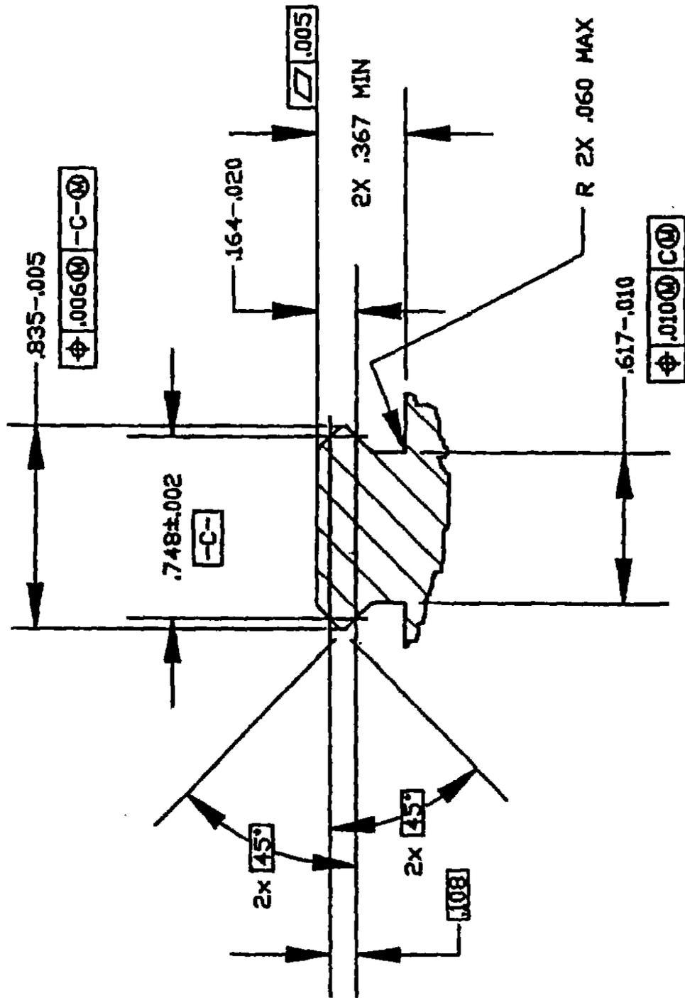
FIGURE 1. ACCESSORY MOUNTING RAIL PROFILE
